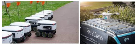
Figure: Autonomous robots and drones for parcel delivery [4,5].
